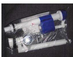
Your local home repair or hardware store can assist you with most of the parts. The fill valve is a short style, the flapper valve is standard 2 1/4". You may need to cut the fill tube so measure the old one when the time comes. The tank-to-bowl gasket (s) is standard. These parts last a long time but you may want to keep this in a file somewhere to make it easy in 10 years when you have to replace them just like in any other toilet.
